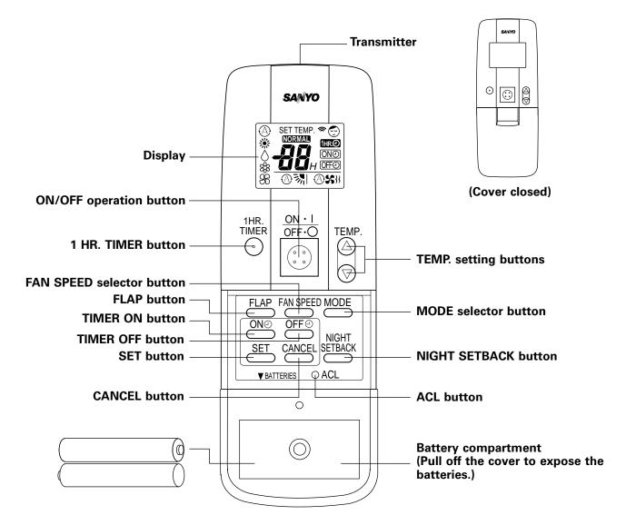
The illustration above pictures the remote control unit after the cover has been lowered and removed.
